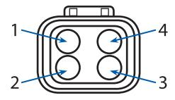
**Pin number 2** (white/black): Low pressure switch return. The switch has a 2.49k ohm resister built into the header; with a full charge of refrigerant the switch is in the open position. If the pressure switch closes due to the pressure dropping below 10psi or a loss of refrigerant, the A/C clutch will disengage. If wire is disconnected or opened, the control module will disengage the A/C clutch and will activate the red LED to blink four consecutive times.
