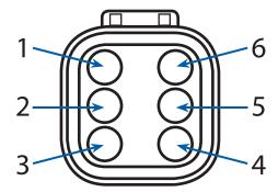
Pin number 2 (red): Control module supply voltage, ignition switched. If voltage drops below 10.0 volts, LED will not illuminate. Low voltage signal is also detected in this circuit. This can be caused by a defective alternator, discharged batteries or excessive electrical loads. This diagnostic is self-clearing, the blink code is displayed only while low voltage is present. If wire is disconnected or has an opened circuit, system will not function.
