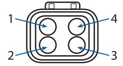
Pin number 2 (white/black): Low pressure switch return. The switch has a 2.49k ohm resister built into the header; with a full charge of refrigerant the switch is in the open position. If the pressure switch closes due to the pressure dropping below 10psi or a loss of refrigerant, the A/C clutch will disengage. If wire is disconnected or opened, the control module will disengage the A/C clutch and will activate the red LED to blink four consecutive times.
